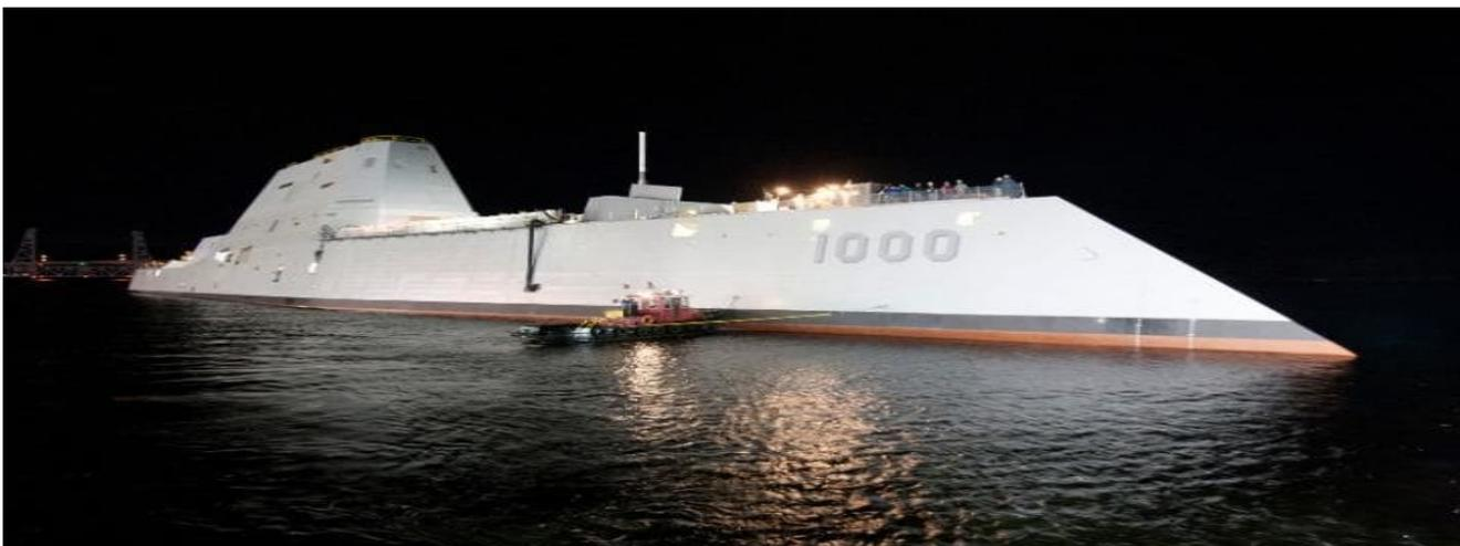
The ship has electric propulsion, new radar and sonar, powerful missiles and guns, and a stealthy design to reduce its radar signature.
